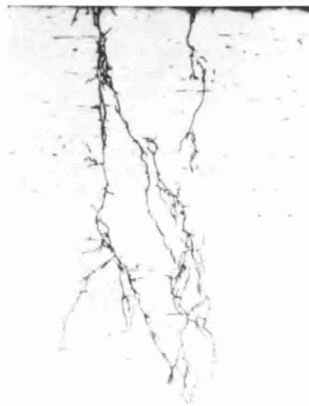
Fig. 11 SCC of AISI type 304 austenitic stainless steel. As-polished. 100x
