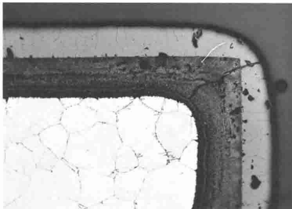
Fig. 18 Multilayer oxide scale formed on Co-10Cr alloy at 1100^\circ\text{C} ( 2012^\circ\text{F} ). Outer layer is CoO; inner (mottled gray) layer is CoO containing dissolved chromium and particles of Co-Cr spinel. The chromium level in this alloy is insufficient to form a fully protective \text{Cr}_2\text{O}_3 scale. Courtesy of I.G. Wright, Battelle Columbus Division
