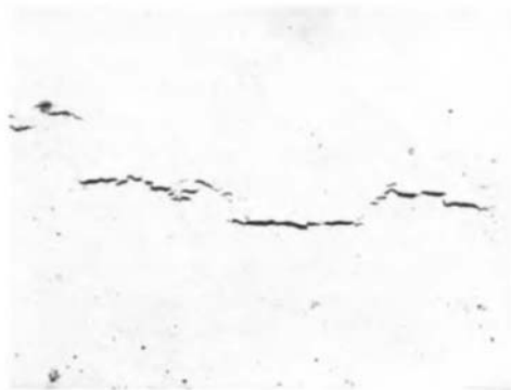
Fig. 1 Hydrogen-induced cracking in a linepipe steel. 30x
